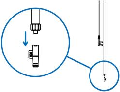
Remove biopsy valve cover or plug from scope Throw out connector and all connector parts Lift scope off scope manager
