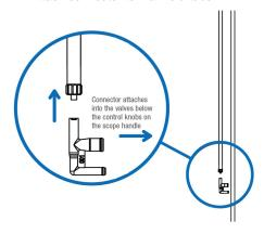
3. Insert connector into suction and air water valve ports below control knobs on the scope
