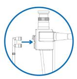
4. If your scope has a water jet port, attach luer coupler or plug to manifold auxiliary water tube, and then attach into water jet port on scope by screwing or inserting it into port
