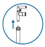
For scopes with a water jet port, remove luer coupler or plug from water jet port on scope, and then remove from manifold auxiliary water tube
