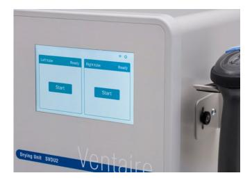
The main screen uses color and a timer to show the drying process.
