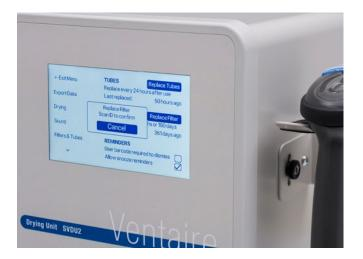
To snooze a notification, select "Allow snooze reminders." To require users to scan the barcode on their ID badge to dismiss the notification screen, select "User barcode required to dismiss."
