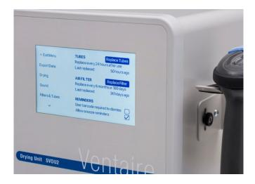
The drying unit will display reminders to replace the tubes and air filter. To change the reminder notification screens, select Filter & Tubes. Administrators can require that users scan the barcode on their ID badge to dismiss a reminder notification and/or set the snooze option for the notification, which allows the user to complete one additional drying cycle.
