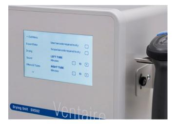
The drying unit is preconfigured with default settings for drying durations, but it is the responsibility of those using the system to determine drying durations based on the organization's guidelines and/or the guidelines provided by the endoscope manufacturer.
