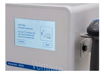
The user can change the drying cycle duration by selecting "+" or "-" until the desired duration is reached, and then select Start or make an additional scan of either the barcode on an ID badge or scope to initiate drying.
