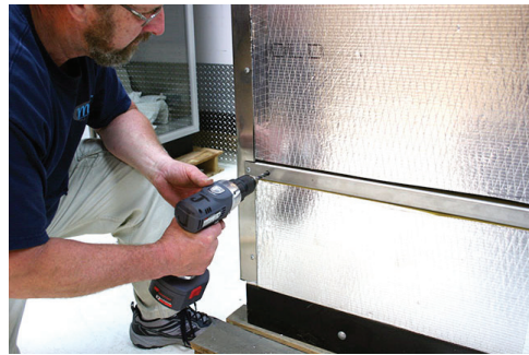
Figure 11: Drill holes on both sides and deburr
