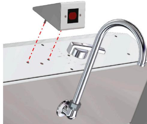
Figure 14: Attach IR sensor housing to header
