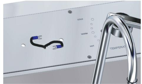
Figure 9: Feed wires through center hole
