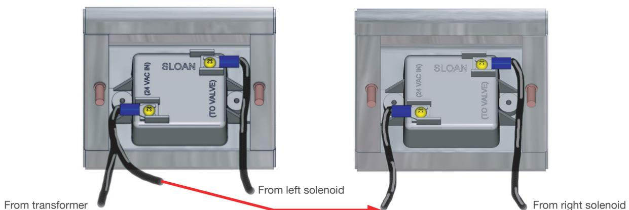
Figure 12: Connect 3 wires - left IR sensor
