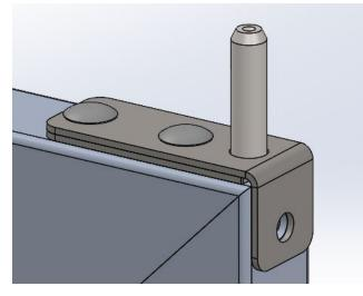
10. Using the 3/16" drill bit, drill a hole into the side door frame through the open hole of the door hinge assembly
