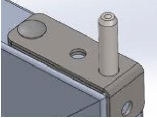
8. Using the 3/16" drill bit, drill a hole in the door frame through the top open hole of the door hinge assembly
