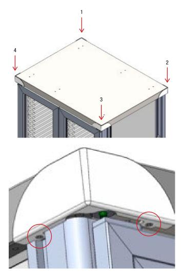
If replacing hinges on a Roam 4 cart, remove the 2 screws from each of the 2 top center trim pieces using a Phillips screwdriver or driver bit with extension. Set aside the center trim pieces and screws
