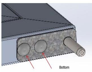
6. Set the bent hinge plate on the flat hinge plate with stud so that the stud goes through the large hole on the bent hinge plate
