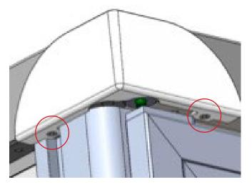
For a Roam 4 cart, attach the 2 top center trim pieces by fastening the 2 screws for each center trim piece using a Phillips screwdriver or driver bit with extension
