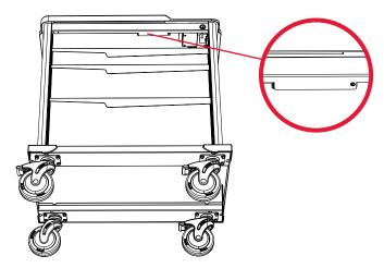
Pull out battery pack holder and remove battery pack
