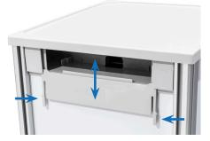
To replace the batteries, open the battery door and lift and remove the battery pack from the cart. Replace the batteries with 8 C-cell batteries (alkaline recommended), and then put the battery pack back into the cart. Slide the battery door up until it clicks into place.
