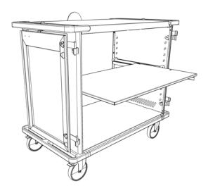
3. Remove shelf slides by pulling slide up and toward you at a 45 degree angle.
