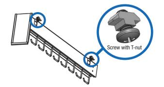
4 screws with T-nuts, 2 in front and 2 in back
